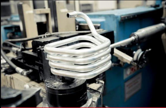
Pipe bending and end forming
